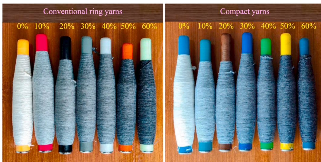
Fig. 10. Ring bobbins of 16 Ne (36.9 Tex) elastic melange yarns produced with varying black recycled cotton% in conventional ring, and compact ring spinning. Black recycle cotton% is mentioned in figure.
