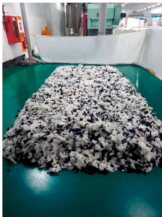
Fig. 4. A representative mixing of recycled cotton: virgin cotton 40:60.
