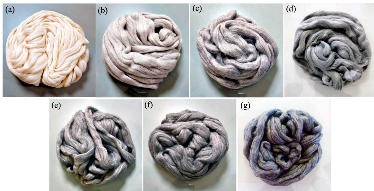
Fig. 5. Finisher draw frame slivers prepared with different blend ratios of recycled cotton:virgin cotton (a) 0:100 (100 % virgin cotton), (b) 10:90, (c) 20:80, (d) 30:70, (e) 40:60, (f) 50:50, and (g) 60:40.
