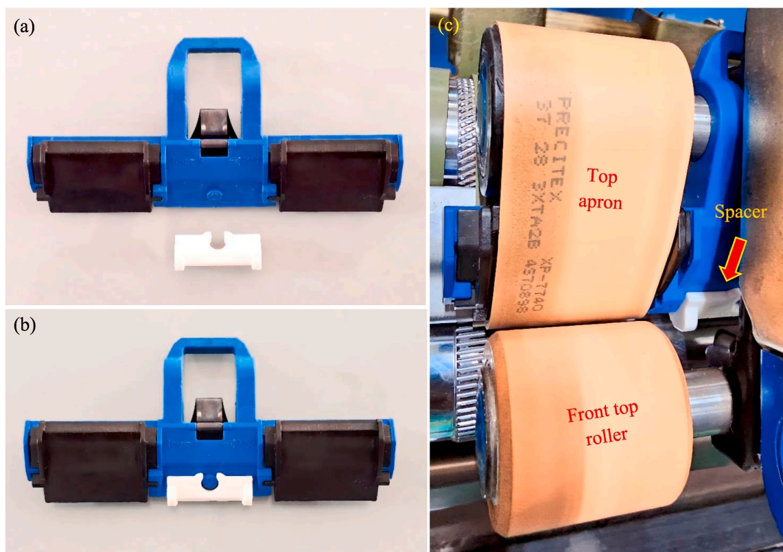
Fig. 7. Traditional spacer used in ring frame: (a) Cradle and spacer, (b) Spacer mounted in cradle, and (c) Spacer (marked by red arrow) drafting zone of ring spinning frame. (For interpretation of the references to color in this figure legend, the reader is referred to the Web version of this article.)
