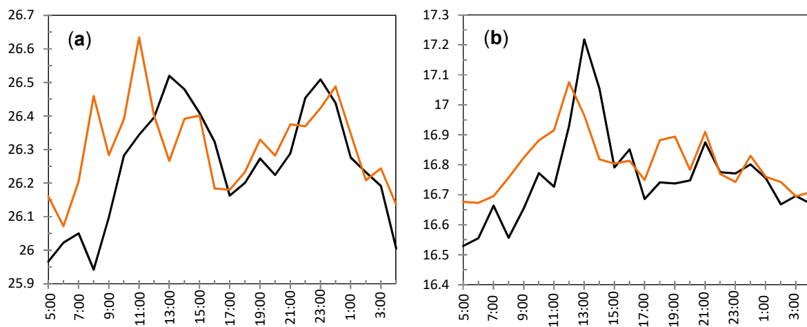
Figure 14. Daily evolution of temperature ( ^{\circ}\text{C} ) for nodes RE5 (brown trajectories) and RE6 (black): (a) averaged for days 1 to 104, (b) averaged for days 105 to 212.
