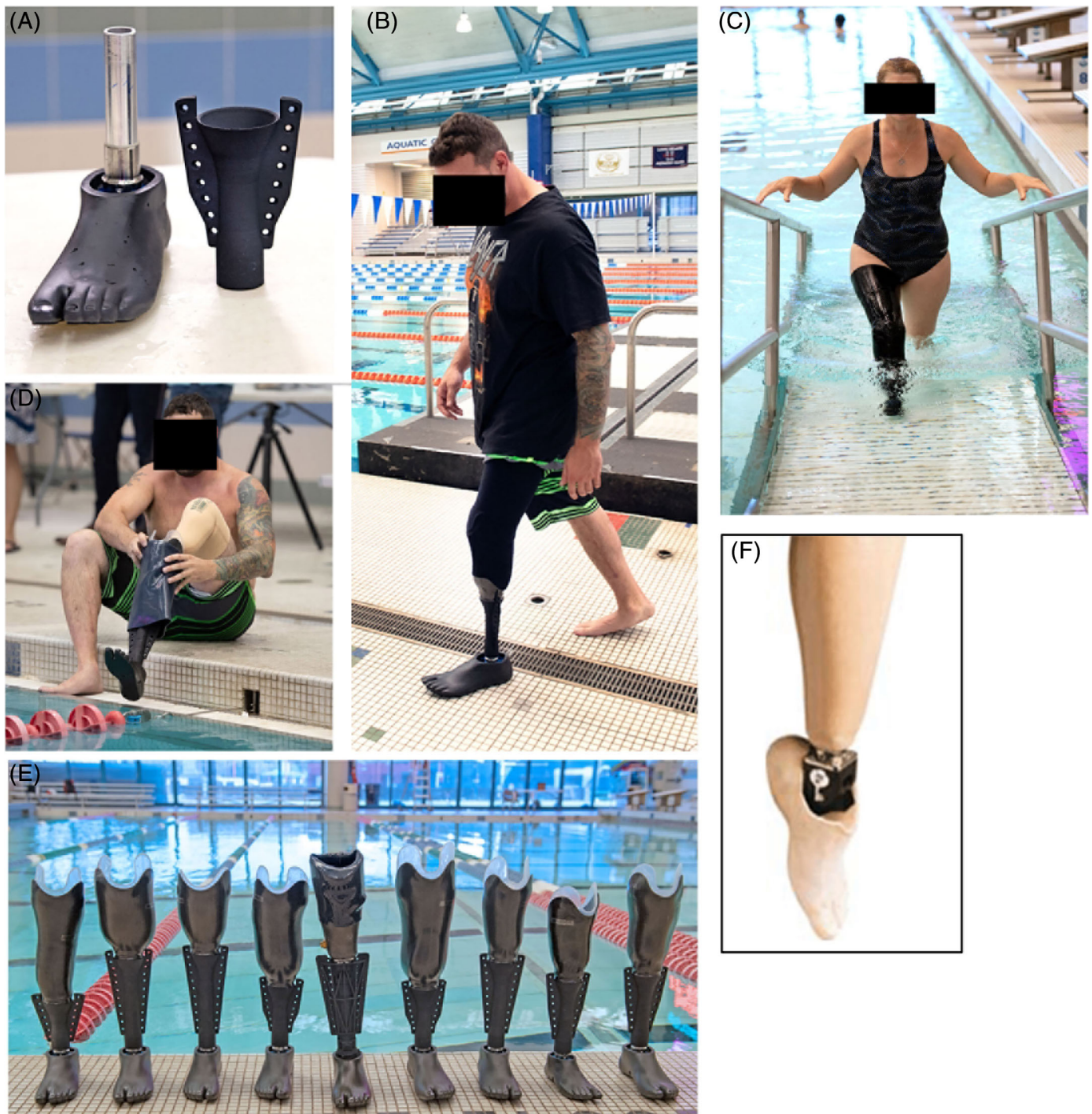
Figure 1. Examples of the novel 3D printed amphibious lower limb prosthesis and its use: (A) The novel 3-D printed amphibious lower limb prosthesis can be used with standard socket and easily assembled. (B) A participant can use the novel 3D printed amphibious lower limb prosthesis for walking over ground or (C) when exiting the pool via a ramp. (D) Donning and doffing the novel 3D printed amphibious lower limb prosthesis is easy and is used with a participant's own standard socket. (E) Each novel device is printed specifically for the user. (F) The Rampro Swim Ankle: The ankle locks into the walking or swimming position as needed (image downloaded from www.rampro.net ).
