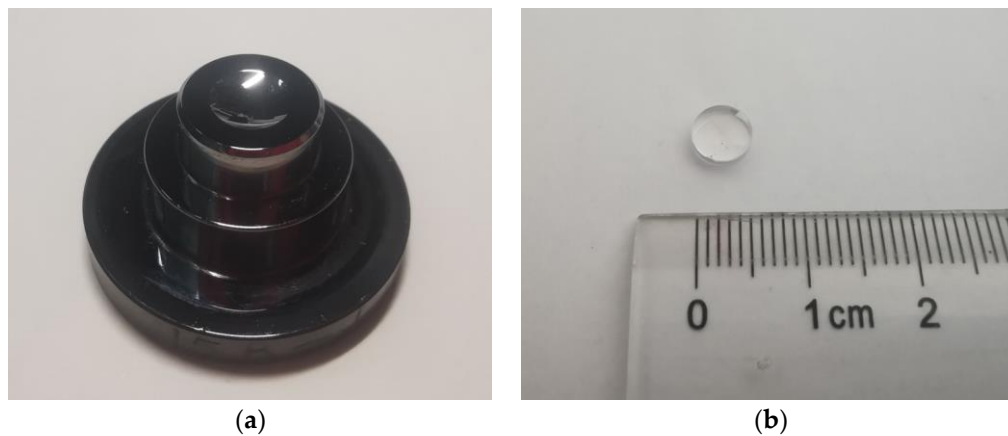
Figure 9. The mold used in PGM experiment and molded glass lens. (a) Fine grinding mold and (b) molded glass lens.
