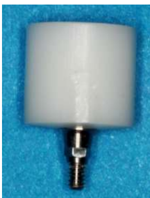
Figure 4: Superstructure cemented to titanium insert
