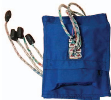
Figure 3. Three-dimensional printed enclosure with 4-accelerometer array.
