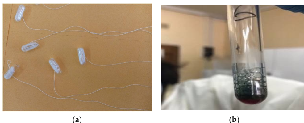
Figure 1. Panel (a) Images of the S-films; (b) an example of the blue colour change occurring on mixing dissolved guaiacum powered, hydrogen peroxide and a solution containing blood.
