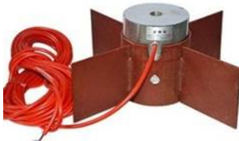
Fig 1. Steel bracing axial force monitoring sensor.
