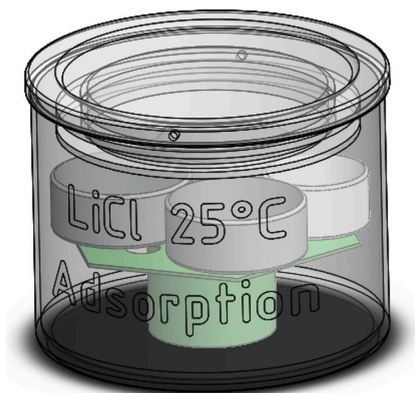
Fig. 1. Hygrostat with three aluminium weighing plates and one with crystal of thymol.
