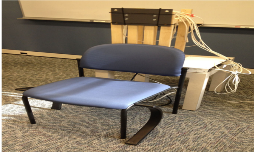
Figure 3: Motion analysis apparatus consisting of the transmitter mounted to a rigid base and a chair for the subjects. The five subjects in this study who were all treated non-operatively at our institution.
