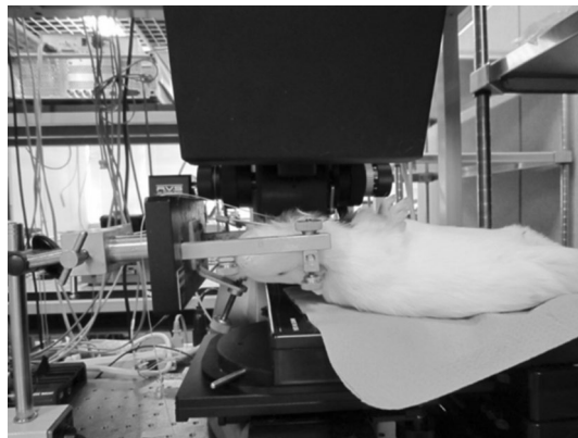
Figure 8. Setting for in vivo OCT imaging. A guinea pig was mounted on the stage with a head holder after the bulla was opened via a ventral approach.
