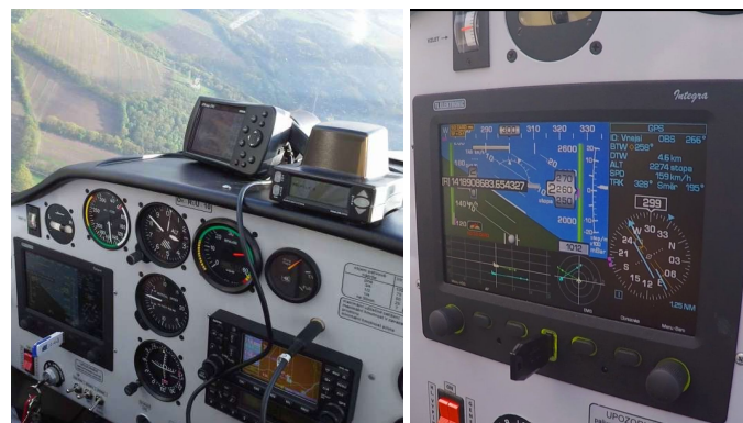
Figure 15. Aircraft pilot panel with the integrated advisory system—built-in EFIS Integra, Zoon PCAS with GPS on the flight panel and the rest of the system integrated under the panel.
