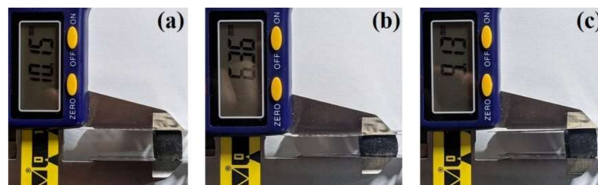
Figure 17. Demonstration of the resilience properties of an equilibrium swollen sample of Co-filled pHEMA-gr-PVP copolymer: (a) initial sample; (b) sample under load; (c) sample after unloading.
