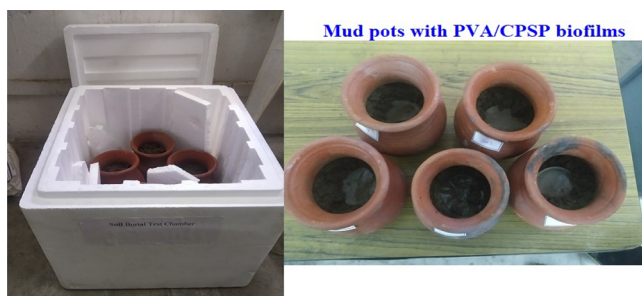
Figure 13. Indoor soil burial test setup.
