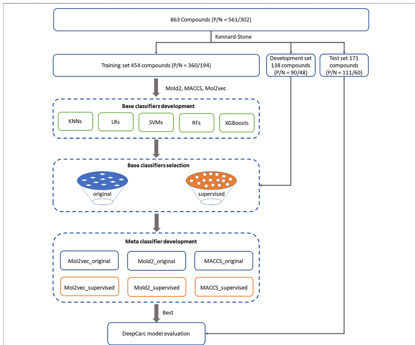
FIGURE 1 | Overall workflow for the DeepCarc model including: (1) Data preparation. 863 compounds were split into training (554 compounds), development (138 compounds), and test (171 compounds) sets based on the Kennard-stone algorithm. (2) Base classifiers development. Five algorithms were used to develop the base classifiers from three different chemical representations, including Mol2vec, Mold2, and MACCS. Two base classifiers selection strategies were employed to select the optimized classifiers for meta classifier development. (3) Meta classifier development. With three chemical representations and two selection methods, six groups of base classifiers, including Mol2vec_supervised, Mol2vec_original, Mold2_supervised, Mold2_original, MACCS_supervised, and MACCS_original. The probability prediction from selected base classifiers was used to train the neural network. (4) Model evaluation. The DeepCarc model was evaluated on the independent test set.
