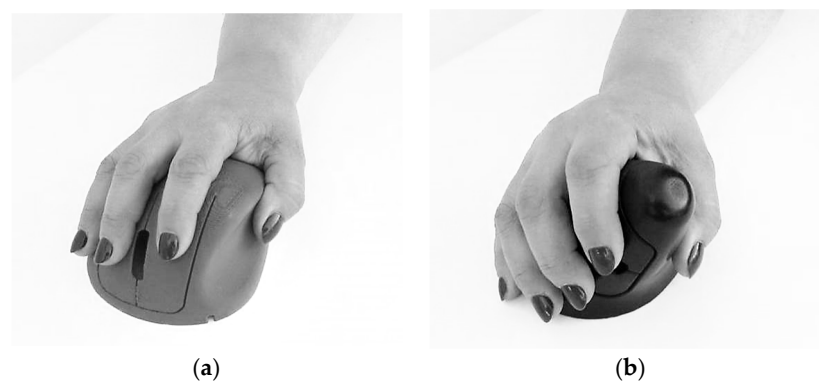
Figure 5. Concept mockups (female adult hand, length 165 mm, width 74 mm, corresponding respectively to 5th and 15th percentile, according to Gordon et al. [26]). (a) ch concept mockup; (b) ci concept mockup.
