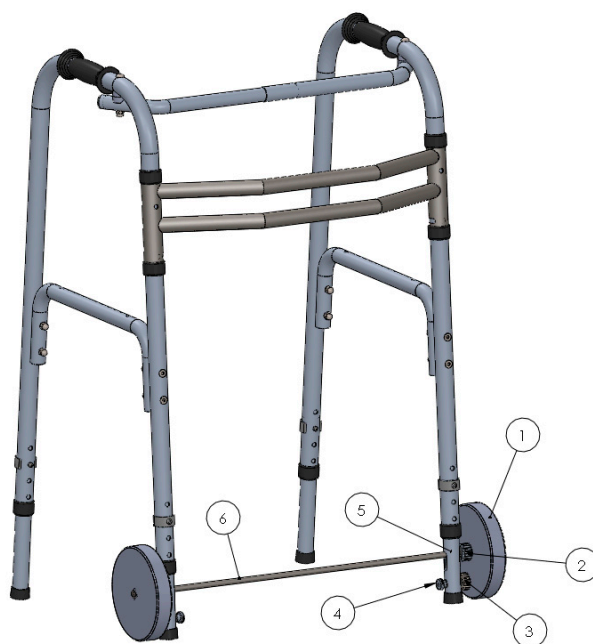
Figure 1. A three-dimensional Computer Aided Design (CAD) model of the walker set and the self-locking mechanism. 1—unidirectional wheels; 2—upper gear wheel; 3—the bottom gear wheel; 4—hand-operated nut; 5—walker's front legs; 6—calibrated steel solid shaft (axis).
