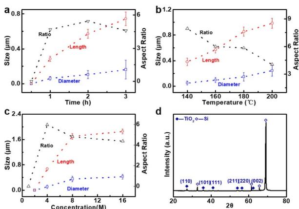
**Fig. 4** (a–c) Statistical schematic of the average diameters, lengths and aspect ratio of the TiO<sub>2</sub> nanorod under different reaction conditions: (a) time, (b) temperature, (c) concentration. (d) The XRD data of the TiO<sub>2</sub> nanorod arrays on the linear template substrate (template is ~5 μm groove and 10 μm array period. Scale bar marked in the figure).
