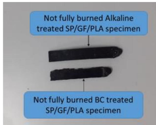
**Figure 10.** Partially burned ASP/GF/PLA and BSP/GF/PLA composites.
