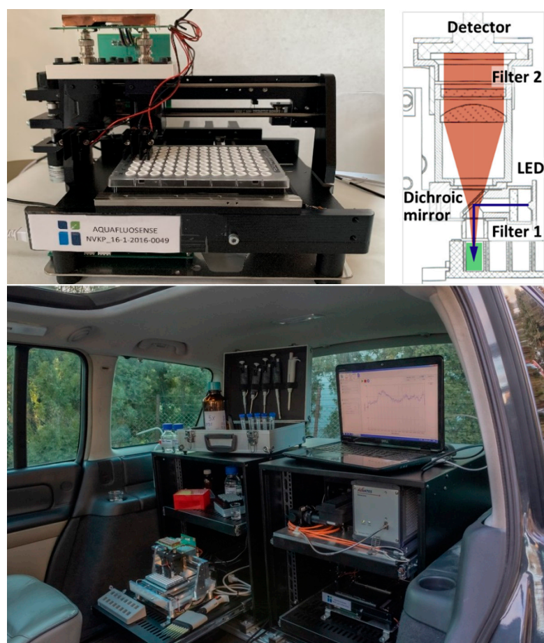
Figure 6. The immunofluorescence module developed in project Aquafloosense and appropriate for zearalenone determination ( top left ). The optical path in the detector head ( top right ). The modular instrumental setup during on site operation in a laboratory motor vehicle ( bottom ).
