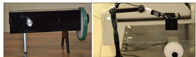
Figure 11: In-house designed and constructed respiratory motion tracking test phantom
