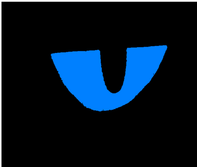
Figure 13. Tomographic slice image after applying simple threshold method.
