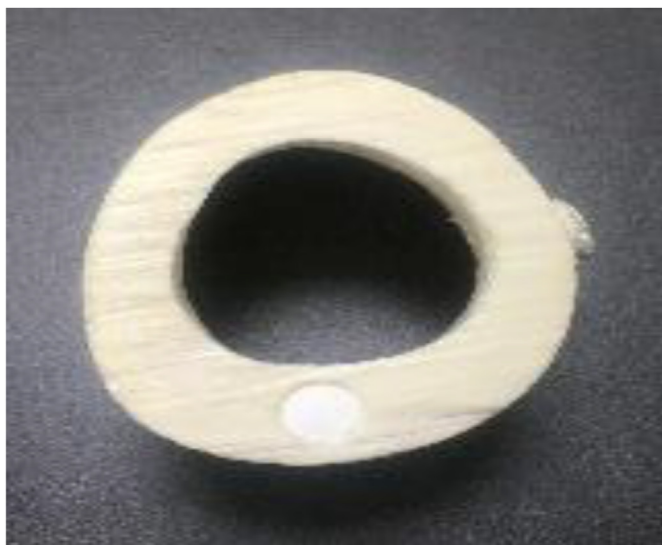
Figure 8. Photographic image of the induced defect with hard cement.
