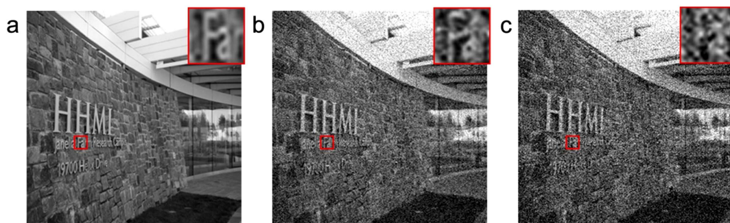
Figure 4 | The analog image transmission experiment. (a) is the original image. (b) is the transmitted image after the iterations. (c) is the result before the iterations. The insets in image (b–c) provide a magnified view of the details for a clear comparison. We thank Dr. Tamir Gonen for providing the original image.
