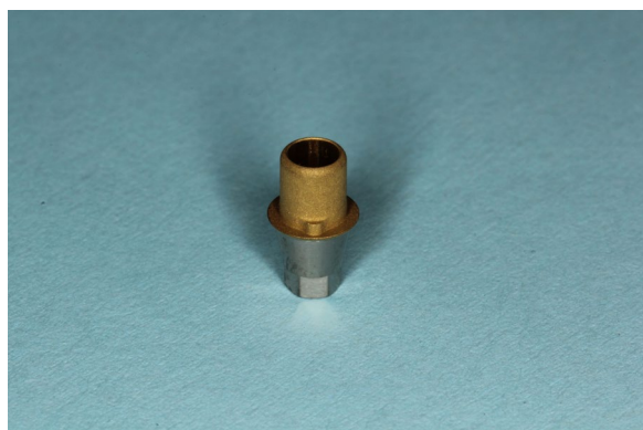
Fig. 1 Prefabricated titanium base of test specimen coated with titanium nitride
