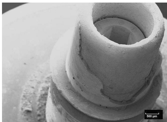
Fig. 8 Scanning electron microscopic view of the titanium base of the specimen shown in Fig. 6 (10 kV, \times 20 , 50 nm). The adhesion of the base is covered by a homogenous layer of the fixation resin
