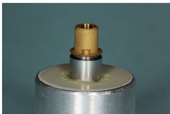
Fig. 3 Test specimen embedded in polyurethane
