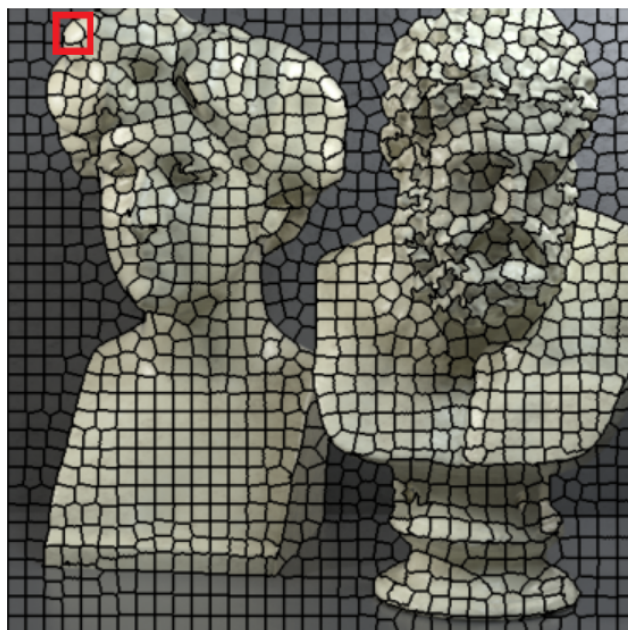
Figure 9. An example of super-pixel segmentation for synthetic LF on dataset Greek, with the number of super-pixels set at 1200. The selection of an arbitrary super-pixel is highlighted in red.
