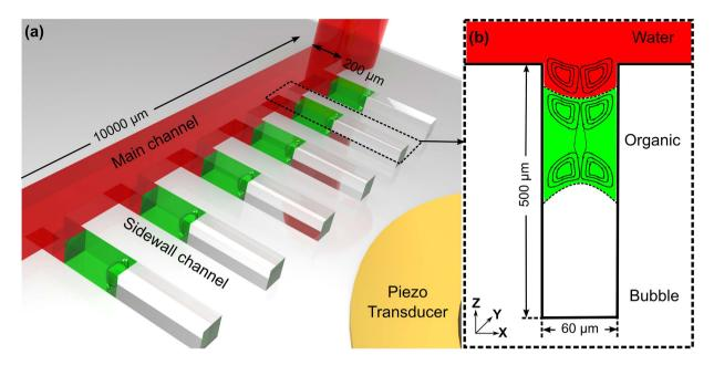
Figure 1. Schematic of the (a) experimental setup and (b) bubble oscillation-induced streaming near the organic-gas surface and near the water-organic solvent interface.
