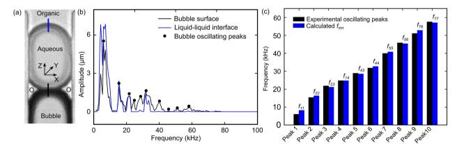
**Figure 4.** (a) Oscillation of the bubble and the liquid-liquid interfaces. The amplitudes of oscillation of the bubble  $(S_1)$  and liquid-liquid interface  $(S_3)$ , are measured along the black line and blue line respectively. (b) Amplitude of oscillation for  $S_3$  and  $S_1$  over a frequency range of 1–100 kHz. The black dots indicate the local amplitude peaks for the bubble. (b) Comparison between the experimentally measured frequencies and the calculated resonant frequencies.
