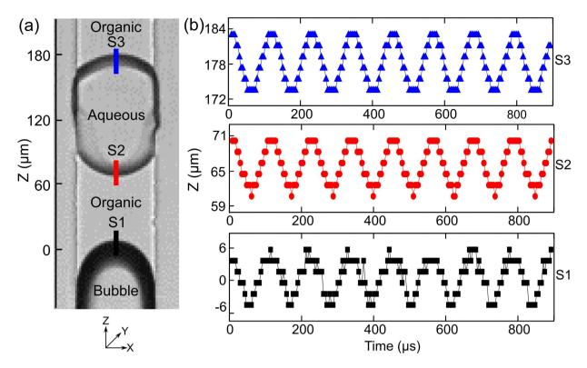
**Figure 3.** (a) Image showing the oscillation of the bubble and the liquid-liquid interface. The position changes in the organic-aqueous  $(S_3)$ , the aqueous-organic  $(S_2)$ , and the organic-air  $(S_1)$  interfaces, is indicated by the blue, red, and black lines, respectively.; (b) The changes in positions of  $S_1$ ,  $S_2$ , and  $S_3$  for an acoustic wave frequency of 10 kHz.
