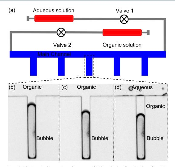
Figure 2. (a) Schematic of the experimental setup to trap bubbles and to form liquid-liquid interfaces inside the T-intersection side cavities;  $(\mathbf{b}-\mathbf{d})$  Sequential flow injection forms an interface between the organic and aqueous phases on top of a bubble.
