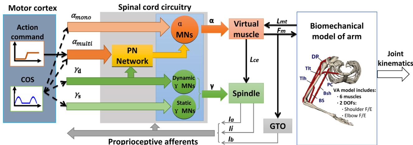
**Figure 1** Corticospinal virtual arm (CS-VA) model used in this simulation study.
