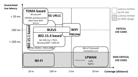
**Figure 2.** Different wireless technologies have different range/latency capabilities. This article discusses the trade-offs in mid-range technologies that could provide coverage of an entire industrial site (black boxes) with sufficiently low latency.
