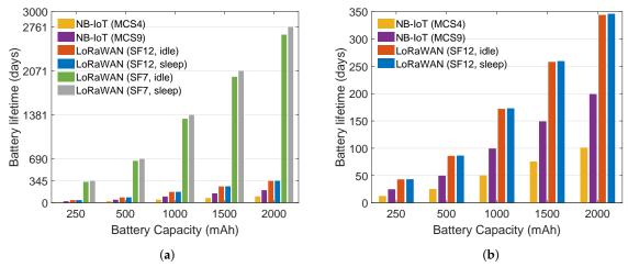
**Figure 6.** Battery lifetime of a device (both radio and microcontroller) transmitting once every 10 min for long-range technologies (<10 km). (b) is a subset of (a) where LoRaWAN SF7 is omitted for clarity.
