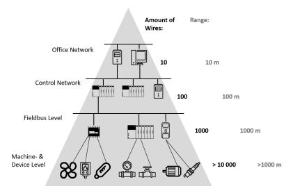
**Figure 1.** Node density exponentially increases from the top (office network/Internet/Intranet) to the bottom (machine- and device-level) in a typical automation system network hierarchy.
