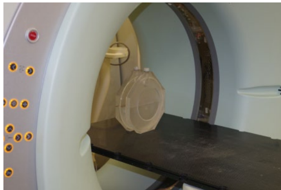
FIG. 3. To check the image rotation angle for axial scans, a phantom half-filled with water is positioned on the tabletop with the center of the phantom close to the isocenter of the CT scanner.
