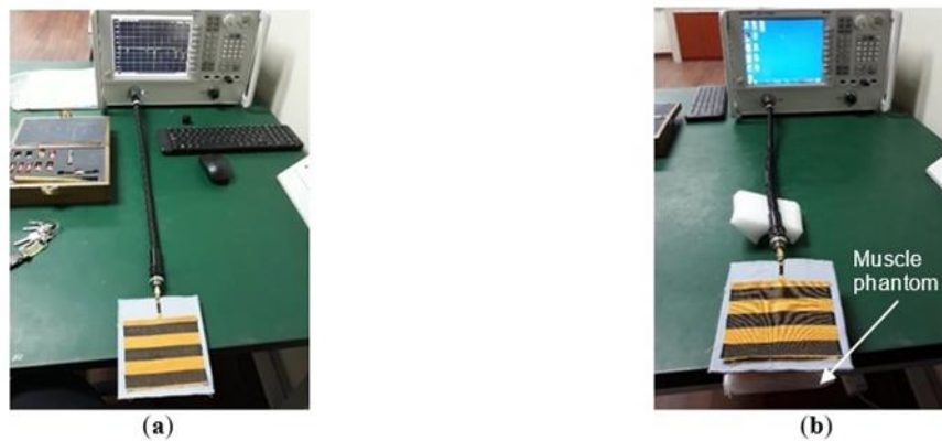
Figure 9. Measurement setup for return loss ( S_{11} ): (a) In free space (Case A); (b) In the presence of the muscle phantom (Case B).
