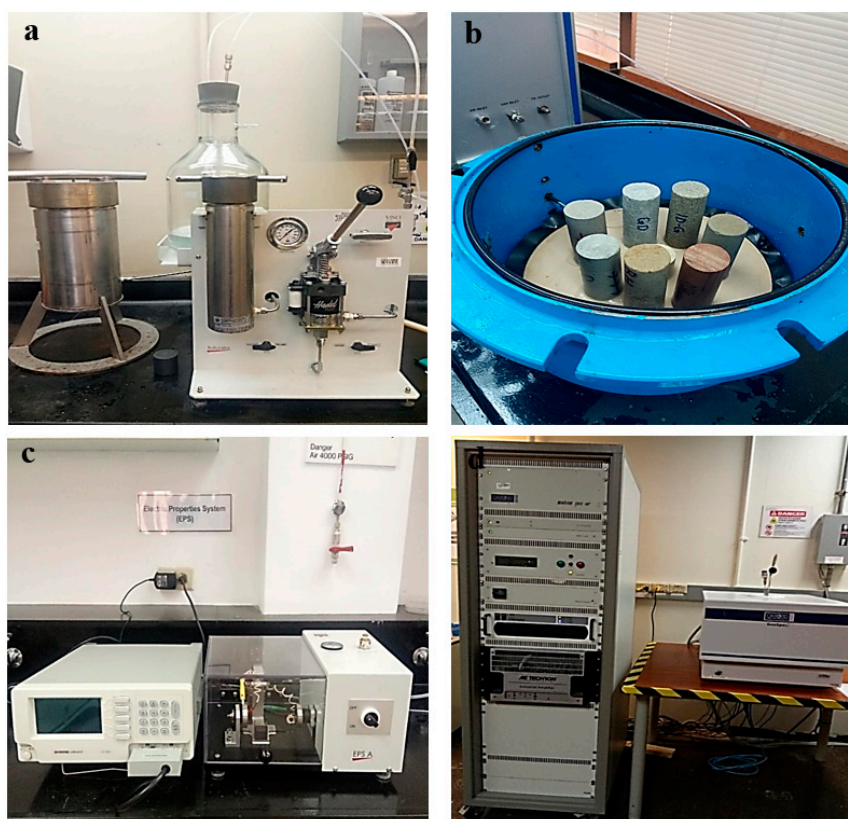
Figure 12. (a) Vacuum saturator; (b) porous plate capillary pressure cell; (c) electrical resistance meter; (d) NMR Geospec 2.1 rock analyzer.
