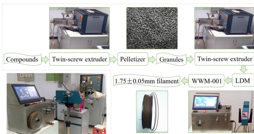
Figure 2. The composite filaments prepared by the “two-step” method.
