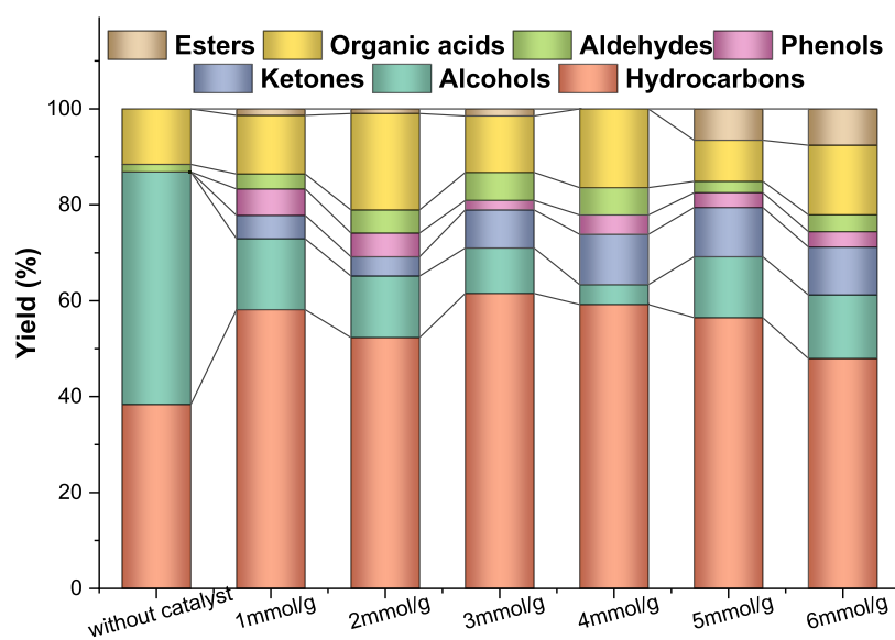
Figure 6. Product categories of shale oil derived from shale aqueous conversion ( 280\text{ }^\circ\text{C} , 4 h, 8 g oil shale, 0.8 g catalysts, 20 mL water).
