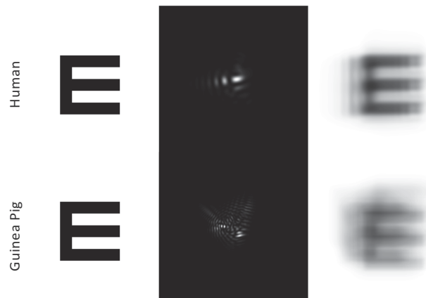
FIGURE 7. Five-arcmin letter E shown alongside PSFs and convolved images for a representative human eye (S09, top row ) and guinea pig eye (#3, bottom row ). Calculations used a 4-mm pupil size and 550-nm wavelength.
