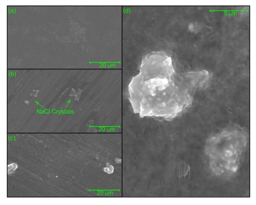
**Figure 8.** Environmental scanning electron micrographs of vancomycin (**a**), bovine submaxillary mucins (**b**) and the complexes resulted from the interaction with vancomycin (**c**,**d**) suspended in 0.1 M PBS (pH 7.0). Aqueous samples were subjected to dehydration in the ESEM sample chamber at operating pressures ranging from ~4 to ~5 Torr. Small globular grains forming the supramolecular aggregate as shown in panel (d), a magnification of lower left panel (c).
