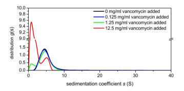
**Figure 4.** Sedimentation coefficient distribution of bovine submaxillary mucin (BSM) and vancomycin at differing mixing ratio. Rotor speed 45000 rpm. 1.0 mg/mL BSM + 0.125 mg/mL (blue line), +1.25 mg/mL (dark green), +12.5 mg/mL (red) vancomycin. The 1.0 mg/mL BSM control is shown in black.
