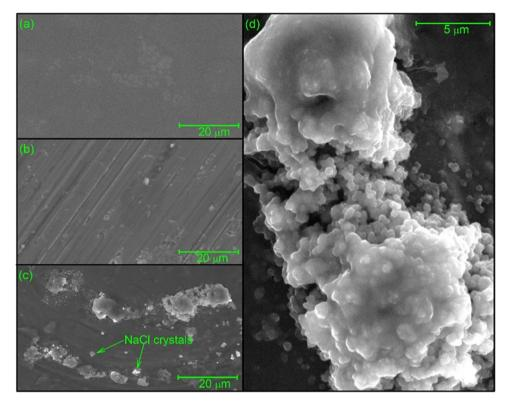
**Figure 6.** Environmental scanning electron micrographs of vancomycin (**a**), pig gastric mucins (**b**) and the complexes resulted from their interaction (**c**,**d**) suspended in 0.1 M PBS (pH 7.0). Aqueous samples were subjected to dehydration in the ESEM sample chamber at operating pressures ranging from ~4 to ~5 Torr. Small globular grains forming the supramolecular aggregate as shown in panel (d), a magnification of lower left panel (c).
