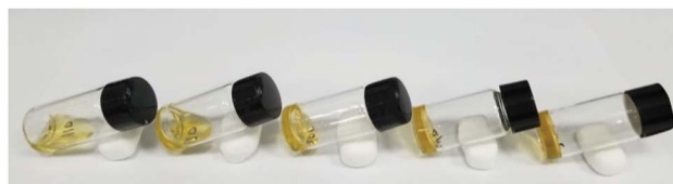
Fig. 6 Photographs of PI/CYC solutions (5 minutes' standing), from left to right corresponding to the volume fractions of 0.077, 0.105, 0.120, 0.139, 0.153, respectively.
