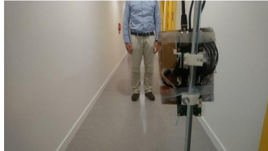
Figure 14. Experiment setup: the preliminary INSPEX prototype is fixed on a white cane; the device tries to detect obstacles (walls, objects, people) in a corridor.
