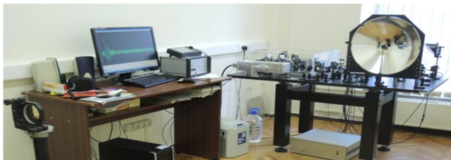
Figure 1. Experimental setup for THz signal measuring at long distance [29].
