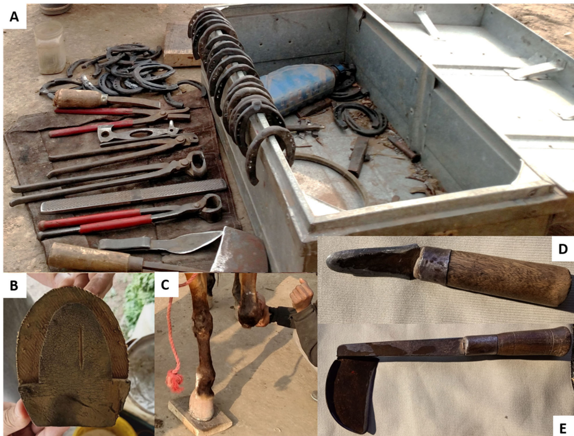
Figure 1. A typical farrier workstation (A) with examples of tools and iron shoes. (B) Rubber shoe insert (C) Plank being used to check hoof balance (D) Hoof knife (E) 'Traditional' hoof knife.
