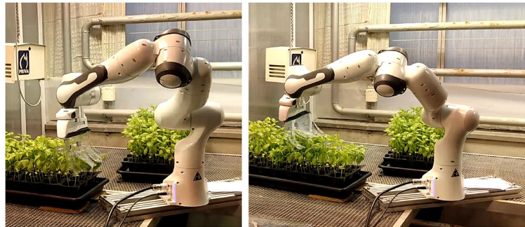
Figure 5. Two types of “robot stroking” motions: dipping (left) and plant-top stroking (right).
