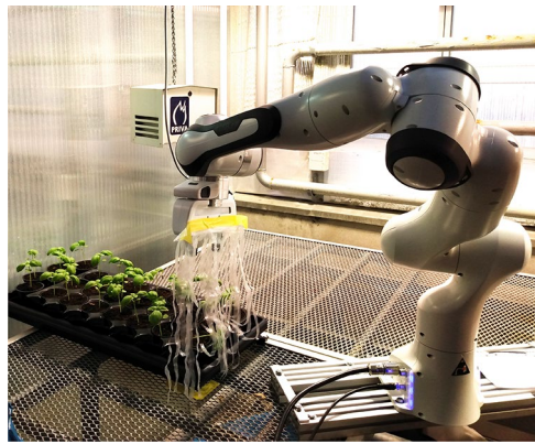
Figure 1. Seven-DoF robotic arm equipped with a stroking end-effector, placed in a commercial-type basil greenhouse setting.
