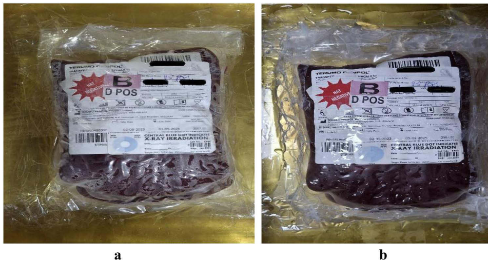
Figure 4 Film indicator before (a) and after (b) irradiation (25 Gy).
