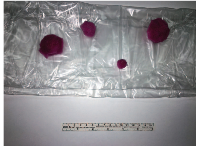
Figure 2. Replications of foam polyps (pedunculated and sessile) secured to the inner lumen of the inner sheath.
