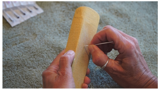
FIGURE 3: Sanding and smoothing the sham needle. The cut end of the handle was smoothed carefully with a sanding block so that no burrs or sharp edges could pierce the skin of the subjects.
