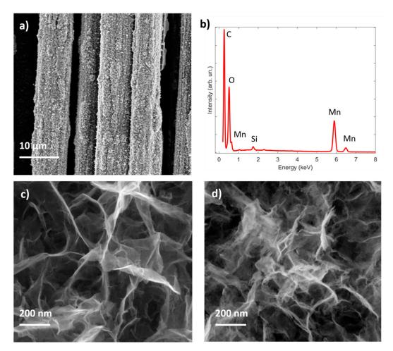
**Figure 1.** (a) Field-Emission Scanning Electron Microscope (FESEM) image of the 2-step electrodeposited manganese oxide showing good coverage of the carbon fibers and (b) representative Energy Dispersive X-ray (EDX) spectrum; higher magnification FESEM images of the 2-step electrodeposited manganese oxide before (c) and after (d) the thermal treatment in  $H_2$ .
