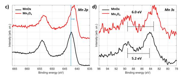
**Figure 2.** (a,b) Show the XRD and Raman spectra of  $MnO_x$  and  $Mn_3O_4$ , (c,d) provide XPS spectra of Mn 2p and Mn 3s regions of manganese oxide before (MnOx) and after (Mn<sub>3</sub>O<sub>4</sub>) the thermal treatment in H<sub>2</sub>.
