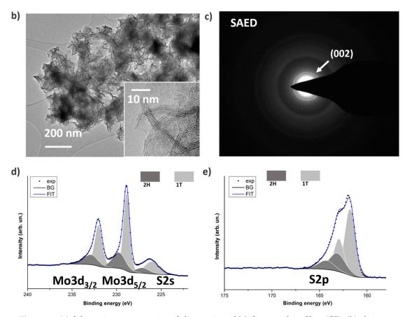
**Figure 3.** (a) Schematic representation of dip-coating of MoS<sub>2</sub> on carbon fiber (CF); (b) shows a low-magnification TEM image of the MoS<sub>2</sub> nanoflakes, while the inset provides a high-magnification image showing the layered structure of the nanoflakes, (c) provides a representative electron diffraction pattern. XPS high-resolution scans of Mo3d/S2s region (d) and S2p region (e) for MoS<sub>2</sub> nanoflakes are presented.
