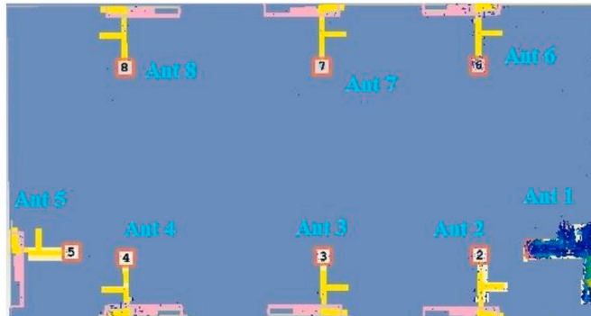
Fig. 7. Surface current distribution on MIMO Antenna due to excitation of Ant-1.
