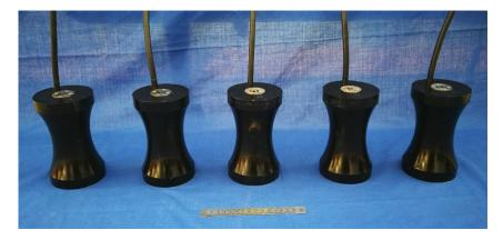
Figure 8. Prototypes of Class I BSFTs with different radii of concave staves.
