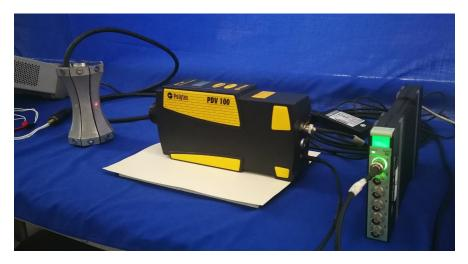
Figure 11. Implementation of vibration test using optical measurement equipment PDV 100 (in air).
