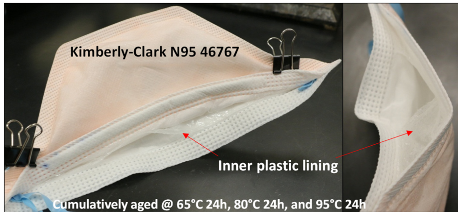
Fig. 8. More pronounced fusing of a specific 'duckbill' mask type (Kimberly-Clark 46767 N95) with these images taken at the final stage after cumulative aging for 24 h each at 65, 80 and 95°C.
