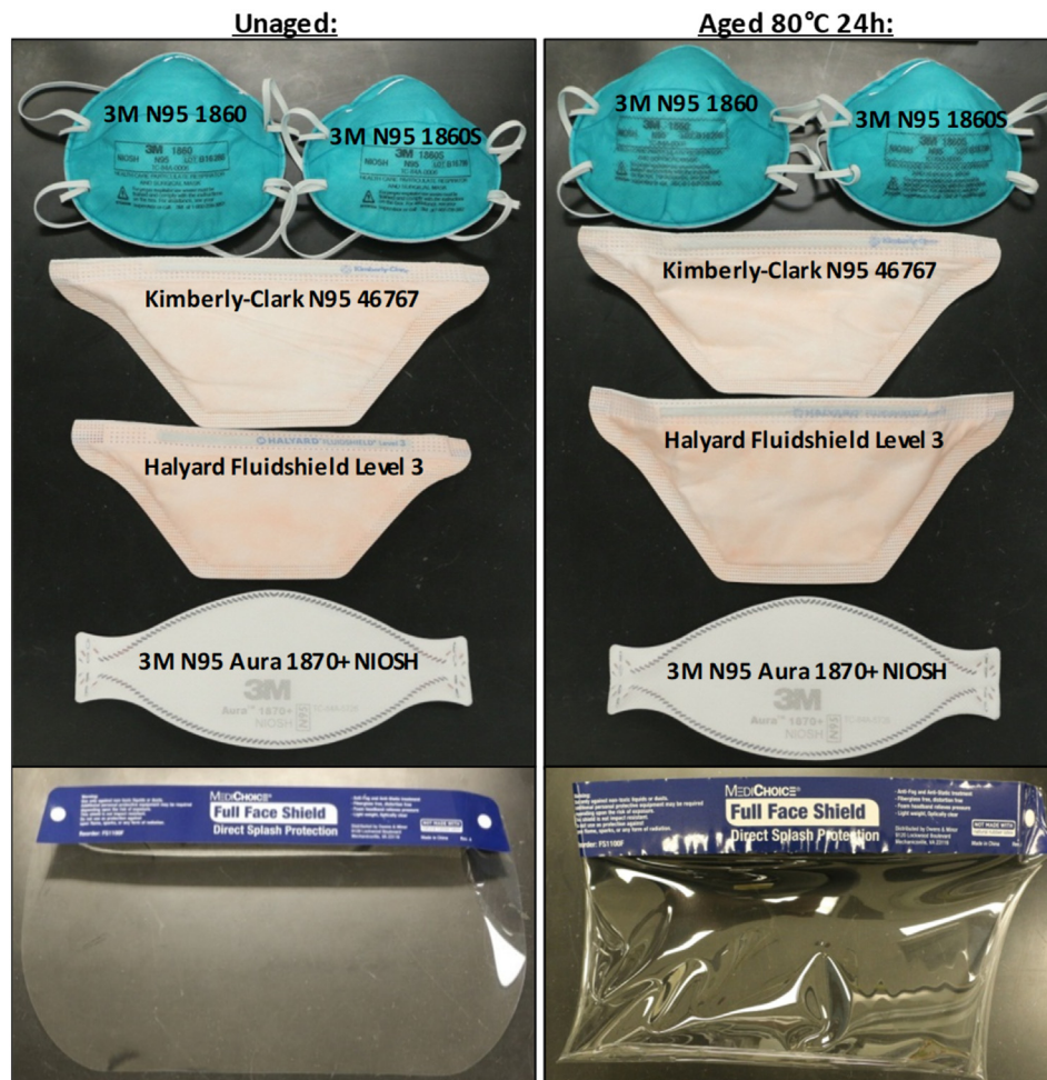
Fig. 5. Different masks thermally aged for 24 h at 80°C before and after exposure.
