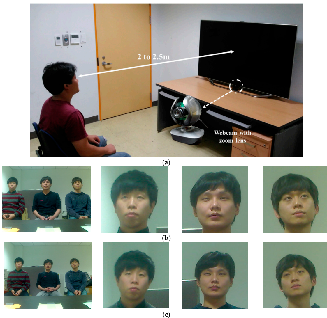
Figure 3. DB1 acquisition environment and obtained images: (a) experimental environment; (b) obtained images (left: Image captured at a distance of 2 m; right: The face images cropped from the images on the left); (c) obtained images (left: the image captured at a distance of 2.5 m, right: the face images cropped from the images on the left).
