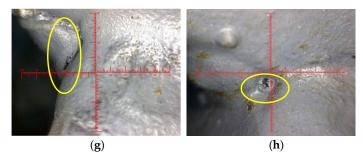
**Figure 7.** Partial enlargement photos of typical weld defect before the fatigue test. (a) South side of the CB/SB1 joint. (b) North side of the CB/SB1 joint. (c) South side of the CB/SB2 joint. (d) North side of the CB/SB2 joint. (e) South side of the CB/SB3 joint. (f) North side of the CB/SB3 joint. (g) South side of the CB/SB4 joint. (h) North side of the CB/SB4 joint.
