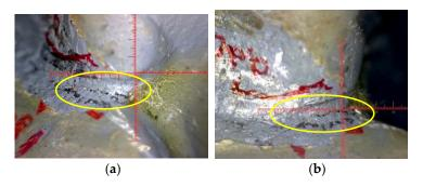
**Figure 8.** Diagram of fatigue cracks of south side of the CB/SB3 joint. (a) 3.2 million cycles. (b) 4.0 million cycles.
