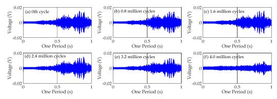
Figure 10. Time domain signals of PZT6 sensor for monitoring south side weld of CB/SB2 joint.
