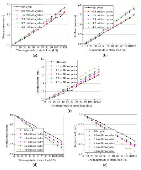
**Figure 9.** Effect of fatigue cycles on static load—displacement curves. (a) Measurement point DI1. (b) Measurement point DI7. (c) Measurement point DI4. (d) Measurement point DI3. (e) Measurement point DI5.
