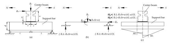
**Figure 12.** Mechanical analysis of CB/SB joint under the test load. (a) Details of the CB/SB joint. (b) Mechanical model of support bar. (c) Bending moment diagram of the support bar.
