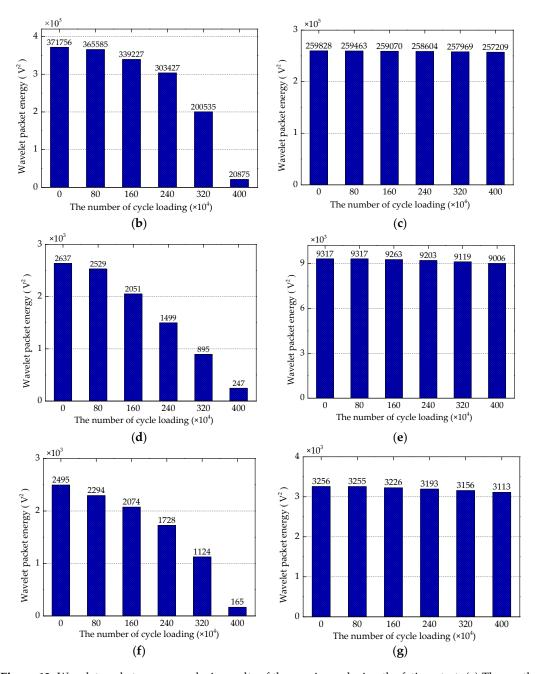
**Figure 13.** Wavelet packet energy analysis results of the specimen during the fatigue test. (a) The south side of CB/SB1 joint. (b) The south side of CB/SB2 joint. (c) The north side of CB/SB2 joint. (d) The south side of CB/SB3 joint. (e) The north side of CB/SB3 joint. (f) The south side of CB/SB4 joint. (g) The north side of CB/SB4 joint.
