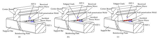
**Figure 2.** The principle of the active-sensing approach. (a) The initial state before fatigue loading. (b) Fatigue crack occurs in the weld throat. (c) Fatigue crack grows along the longitudinal axis of the center beam.
