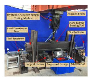
Figure 5. Photo of the experimental setup.
