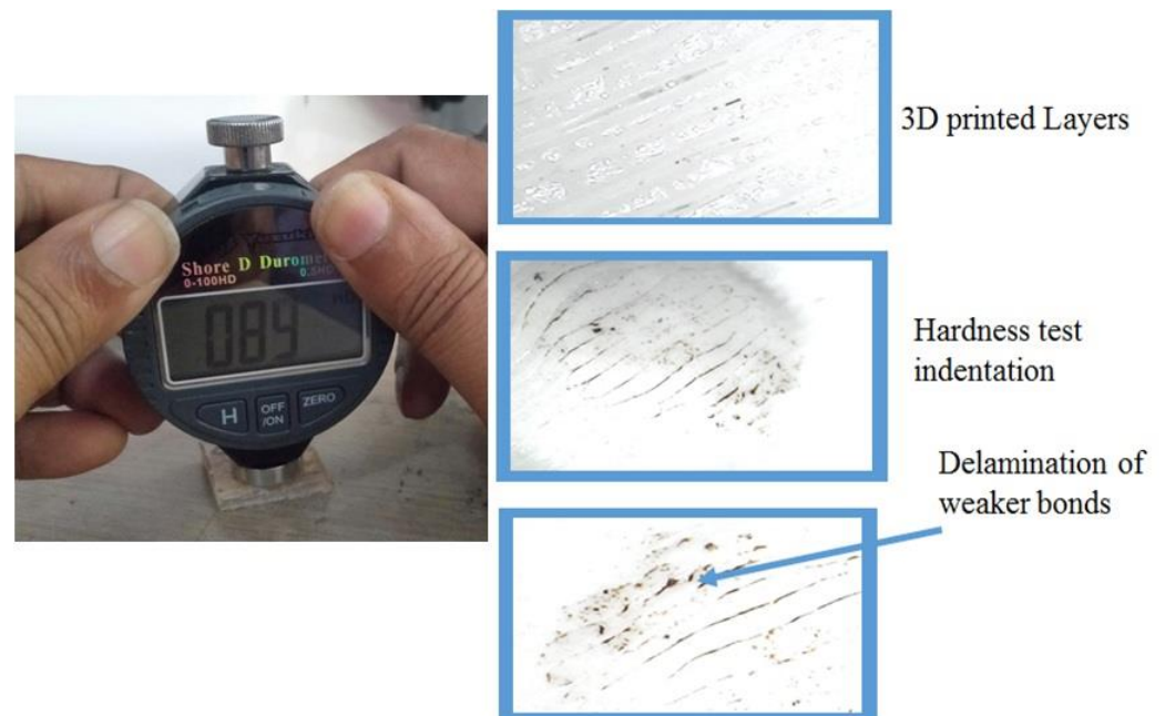
Figure 10. Hardness test setup and delamination of weaker bonds of 3D-printed test specimen.
