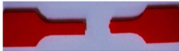
Figure 7. 3D printed ASTM D638 specimen after failure.
