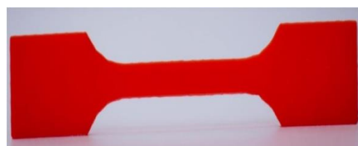
Figure 2. Test Specimen—ASTM D638.
